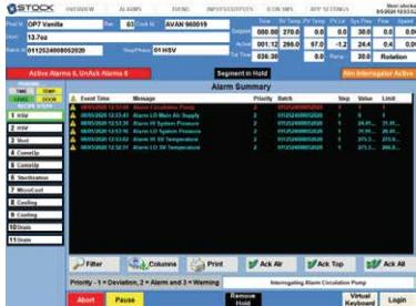
The STOCK™ Alarm Challenge module is available with the STOCK ICON SCADA control system. Designed specifically to test and document all alarms, devices, logic, and critical control factors.
